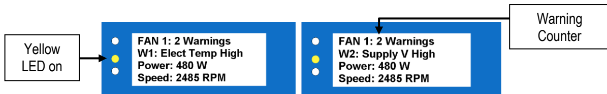
Figure 25 - Example of a first warning on a fan Figure 26 - Example of a second warning on a fan
