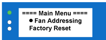
Figure 5 - Main menu display screen on first application of power
