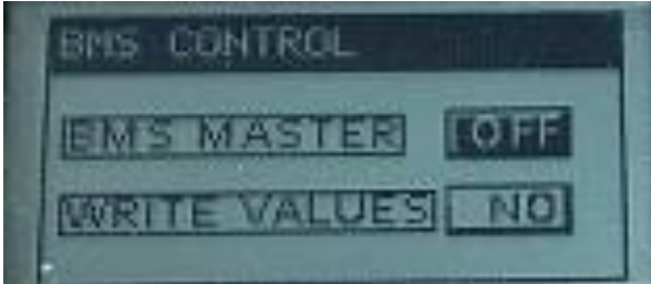
Figure 32: Gateway screen - BMS Control Settings
