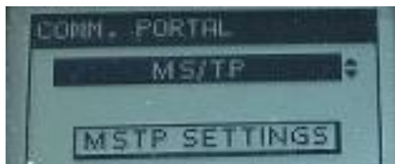
Figure 26: Gateway screen - set MS/TP RS485 communication parameter
