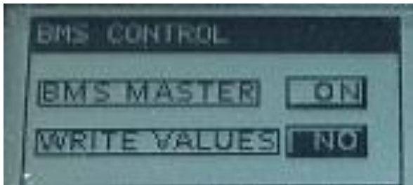
Figure 33: Gateway screen - BMS Control Settings
