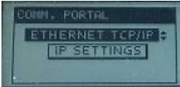
Figure 18: Gateway screen - set Ethernet TCP/IP communication parameters
