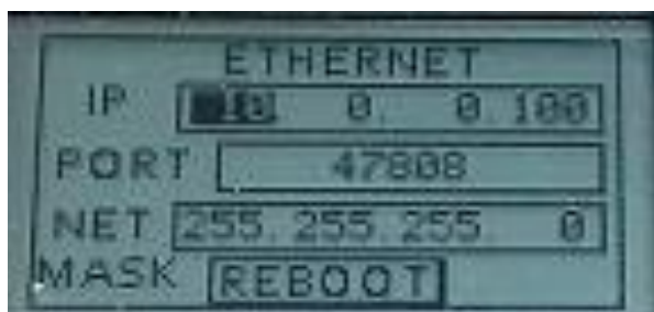
Figure 20: Gateway screen - set Ethernet TCP/IP communication parameters
