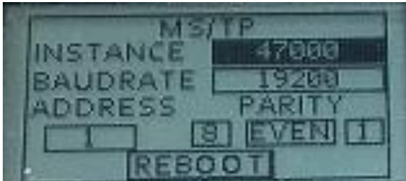
Figure 28: Gateway screen - set MS/TP RS485 communication parameter
