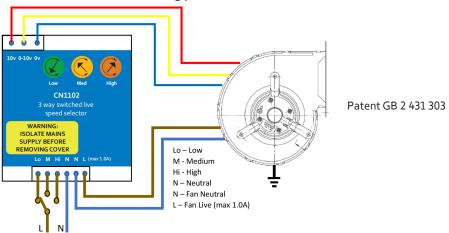
Controller connection for fans with current consumption greater than 1.0A or for an array of fans:
