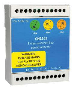
The 3-speed switched live speed selector is designed to allow ebm-papst EC fans with a 0-10v control input to be used with a traditional AC switched live circuit. The selector uses the 10v output and 0v ground reference from the fan control interface. Up to 3 speeds can be selected using the mains input connections. Each speed can be adjusted using trim potentiometers for commissioning purposes.
