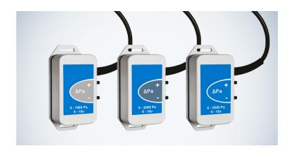
The differential pressure sensor uses a highquality mass flow module to convert the movement of clean air and non-aggressive gases into a 0-10VDC pressure signal. The differential pressure sensor also features a wide power supply range with reverse polarity protection, zero offset, full calibration and temperature compensation (-10°C to +60°C) and has factory calibration for Air and N2.
