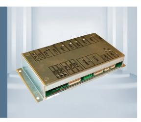
The Thermal Management System (TMS) is a flexible and fully configurable controller that can be used with EC/DC four wire speed controlled fans. Each fan can be individually speed controlled against one of the two temperature sensor inputs. The controller has four Solid State Relays (SSR's) that can be individually configured to give an alarm output against speed or temperature.
