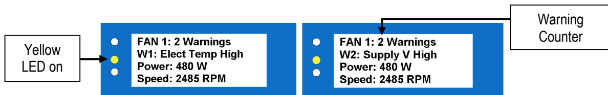
Figure 22 - Example of a first warning on a fan
