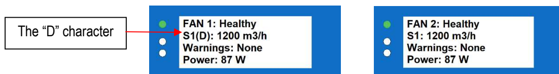
Figure 19 – Fan status screen showing individual sensor readings in m3/h
