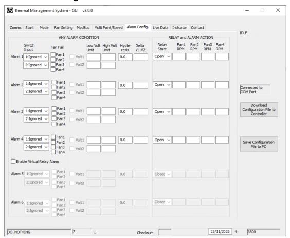
There are 4 standard alarm outputs and two optional additional on the TMS controller (see Enable Virtual Relay Alarms). In an event of specified conditions with the fan(s) and NTC(s) and switch input(s), there can be consequent pre-set action(s). These alarm conditions are configurable within this Tab and consist of:
