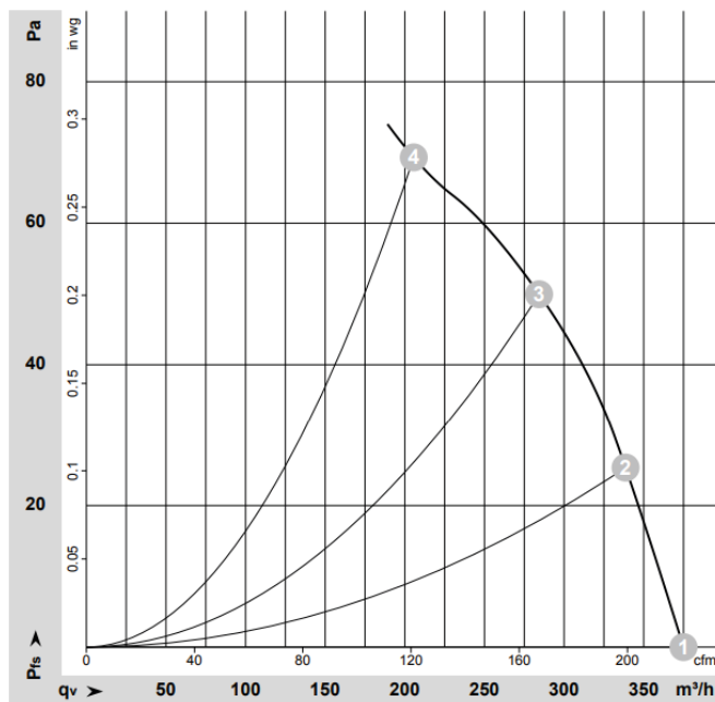
Pressure over air flow at 60Hz
