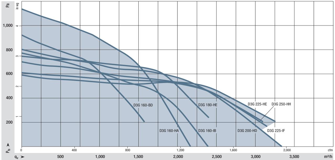
Fan power measurements are carried out on state-of-the-art chamber test rigs. The entire fan unit, consisting of motor, control electronics, and impeller, is measured at varying load states. This ensures that we obtain reliable data, and that you can count on these values being reached when selecting a fan. There are therefore no nasty surprises in store when starting up the fans.
