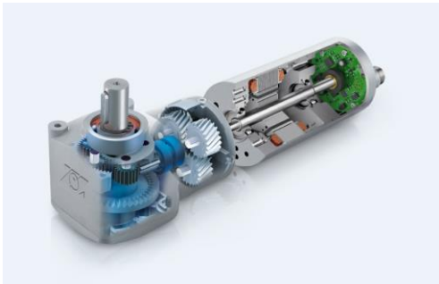
Fig. 1: The involute drive pinion in the crown gearbox is cylindrical in shape and the contact between the pinion and output gear is a rolling contact. Hardly any friction losses occur.
